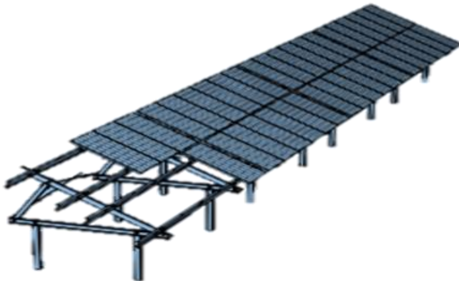
Figure 33 Example of a table (2V) with 2 vertical panels aligned in south orientation
