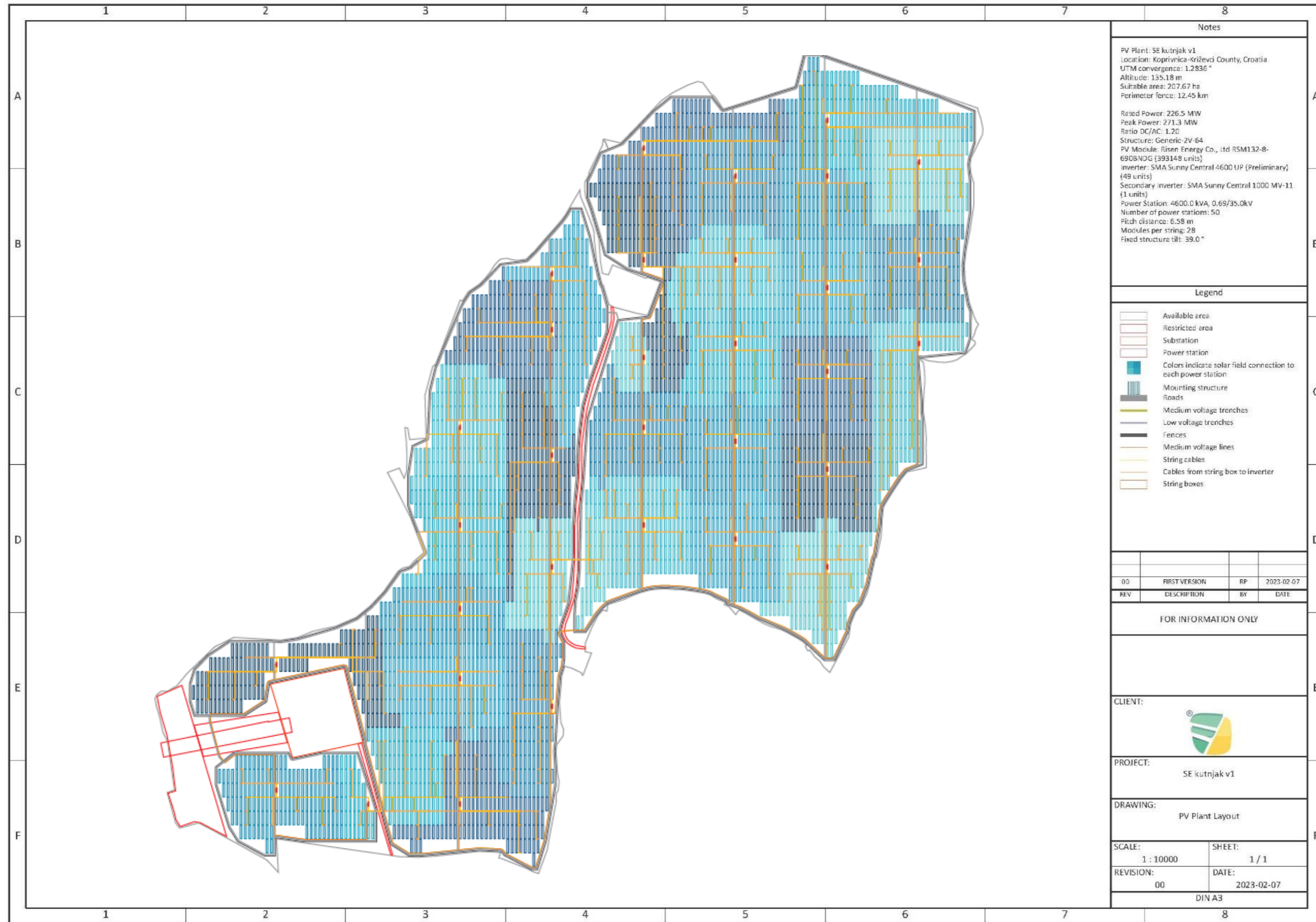
Figure 36 South-4 design with 271 MWdc installed capacity in south orientation – general layout of the panels
